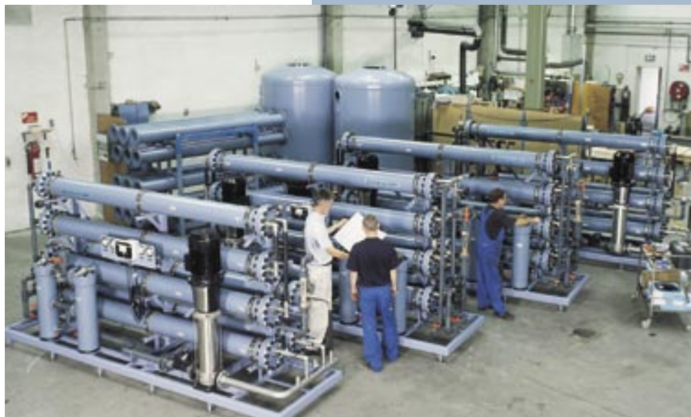
Reverse osmosis plants in process of manufacture for treatment of boiler feed water at pharmaceutical company.
